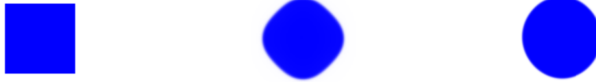
Figure 4: Example of a single solution multi phase separation. Frames from left to right: 0, 400, and 2300 time steps in a 100x100 lu area and depict the density of component one (i.e. [0]).
