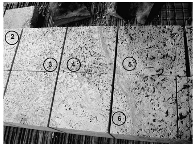
Fig. 2 Cubes (0.3 m) in original position on cutting cart. Note dense laminated layer running through cubes 4, 5 and 6
